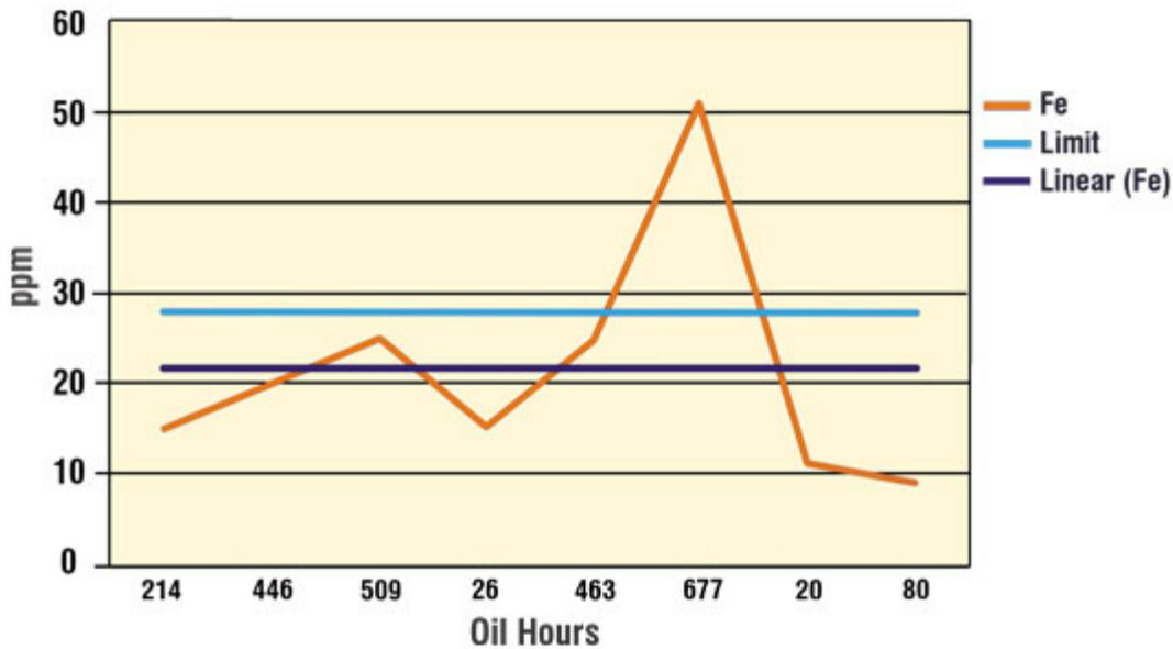
Figure 1. Analysis of increasing wear metals in mineral oils before installing bypass filters
