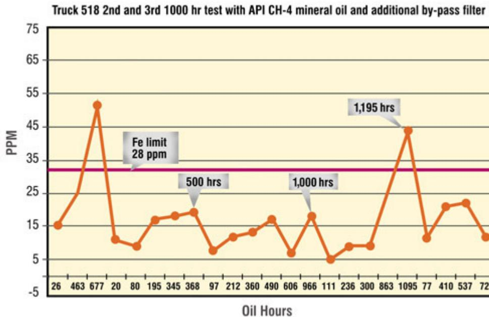
Figure 2. Analysis of wear limits in mineral oil after bypass filter installation
