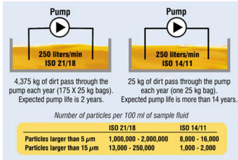
The study showed that bearing and pump life should increase significantly with lower particle concentration.
