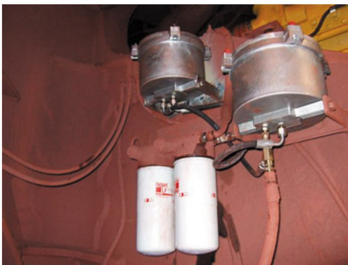
Installing bypass filters was key in extending the service intervals on the haul trucks at the Sishen mine.
