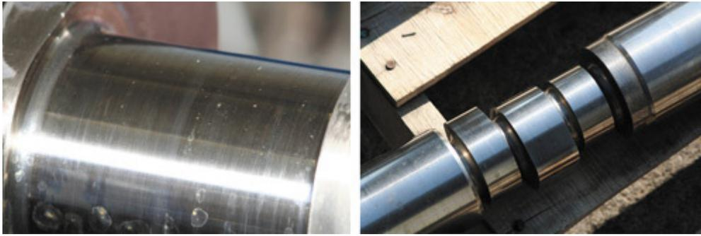
*After 28,000 hours of operation, this crankshaft (left) and camshaft (right) from a haul truck only needed polishing before being reused.*
